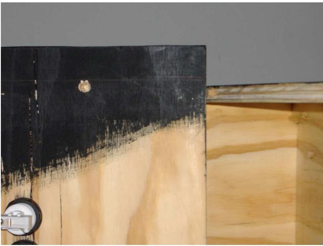
Here is the hole only going though part way from the bottom of the control panel top. Just barely, next to the top, you can see the peg in the top of the side panel of the control box. Please note this picture is sideways, I stood it up on its end to work on it, and for this photo.
