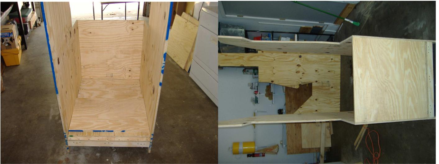
Next is the speaker panel. As of this point, I just added in some basic speakers, with plans about adding in some good speakers in the future. I measured 5 inches in from the sides, and three inches in from the front. This was my center point to drill with a “door knob” drill bit. Once again, I sanded the insides of the holes a little to remove the rough edges.
