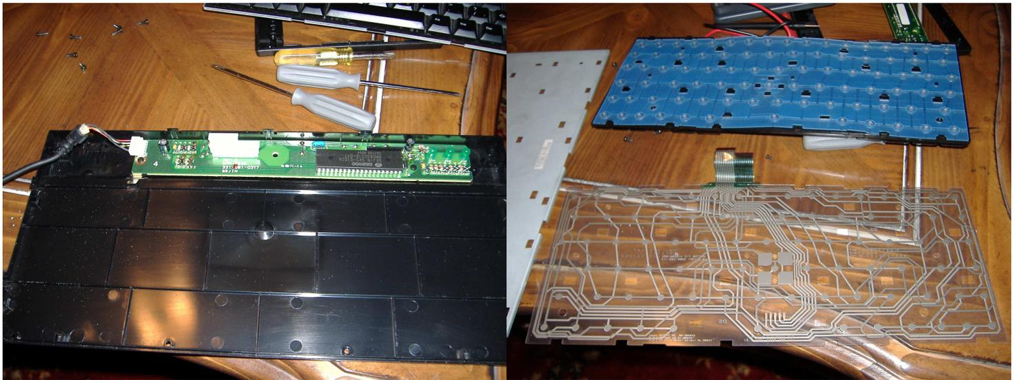
What we need is the circuit board from inside. Also save the keys themselves, and the clear sheets what make up the contacts for the keys. This is the part in the right photo at the bottom.
