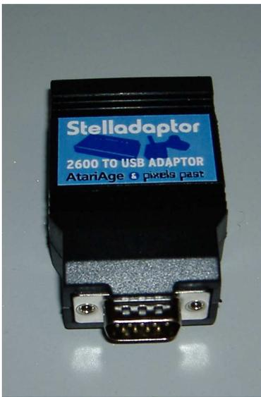
Here is a photo I took of the Stelladaptor. It is the “standard” nine pin joystick connector on one end, and USB on the other.
